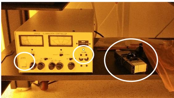
Figure 2: Contact aligner power supply. Circled from left to right are the start button, power switch, and intensity meter.
