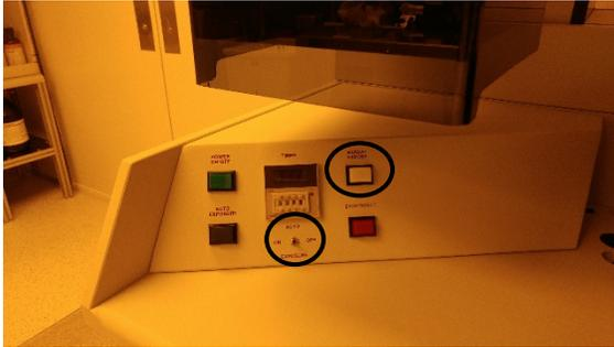
Figure 4: Left side of the contact aligner control panel. Circled from left to right are the auto-exposure switch and manual expose button.
